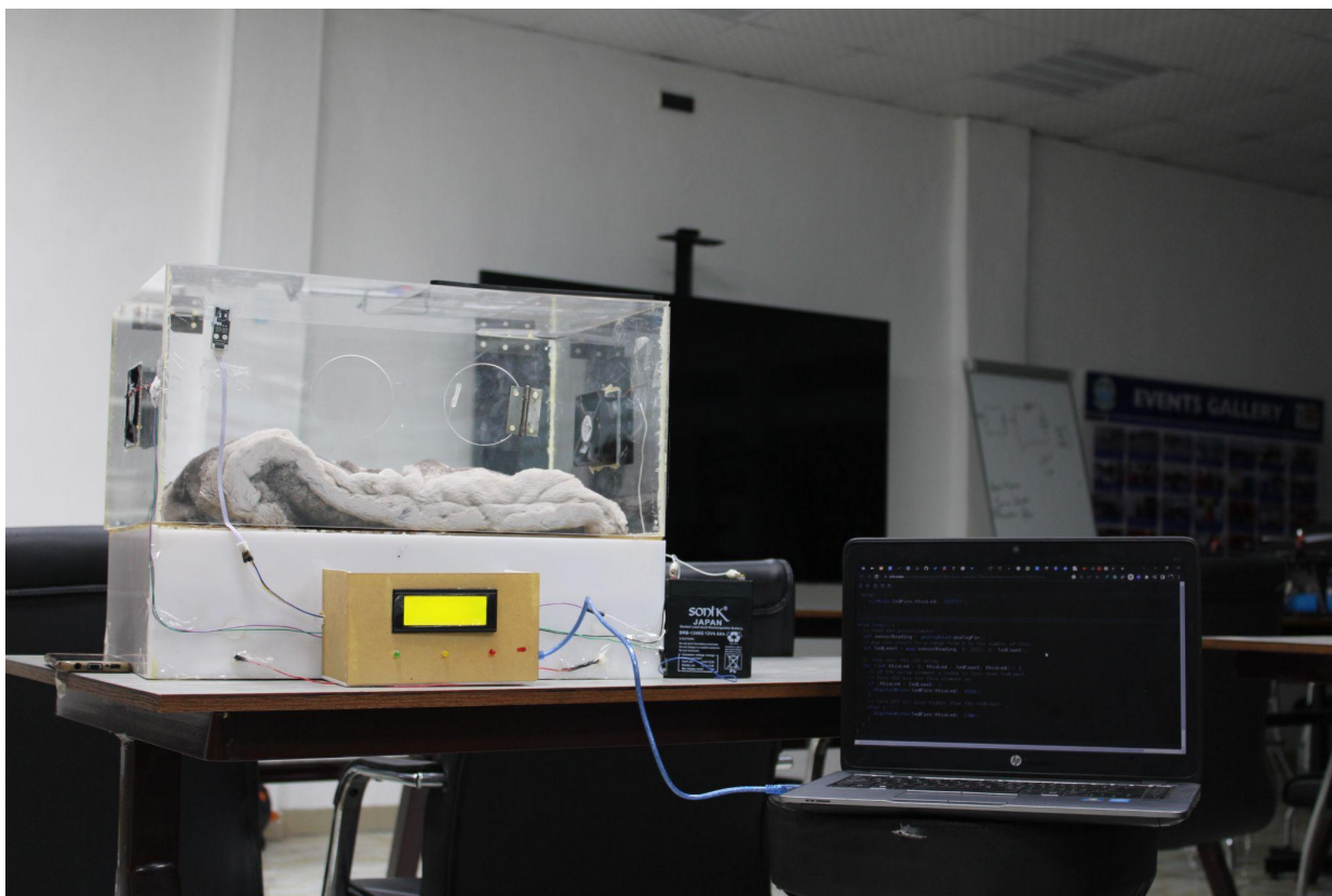
Figure 7. Integrated prototype with the acrylic chamber, ventilation fans, lower thermal compartment and external demonstration hardware.
